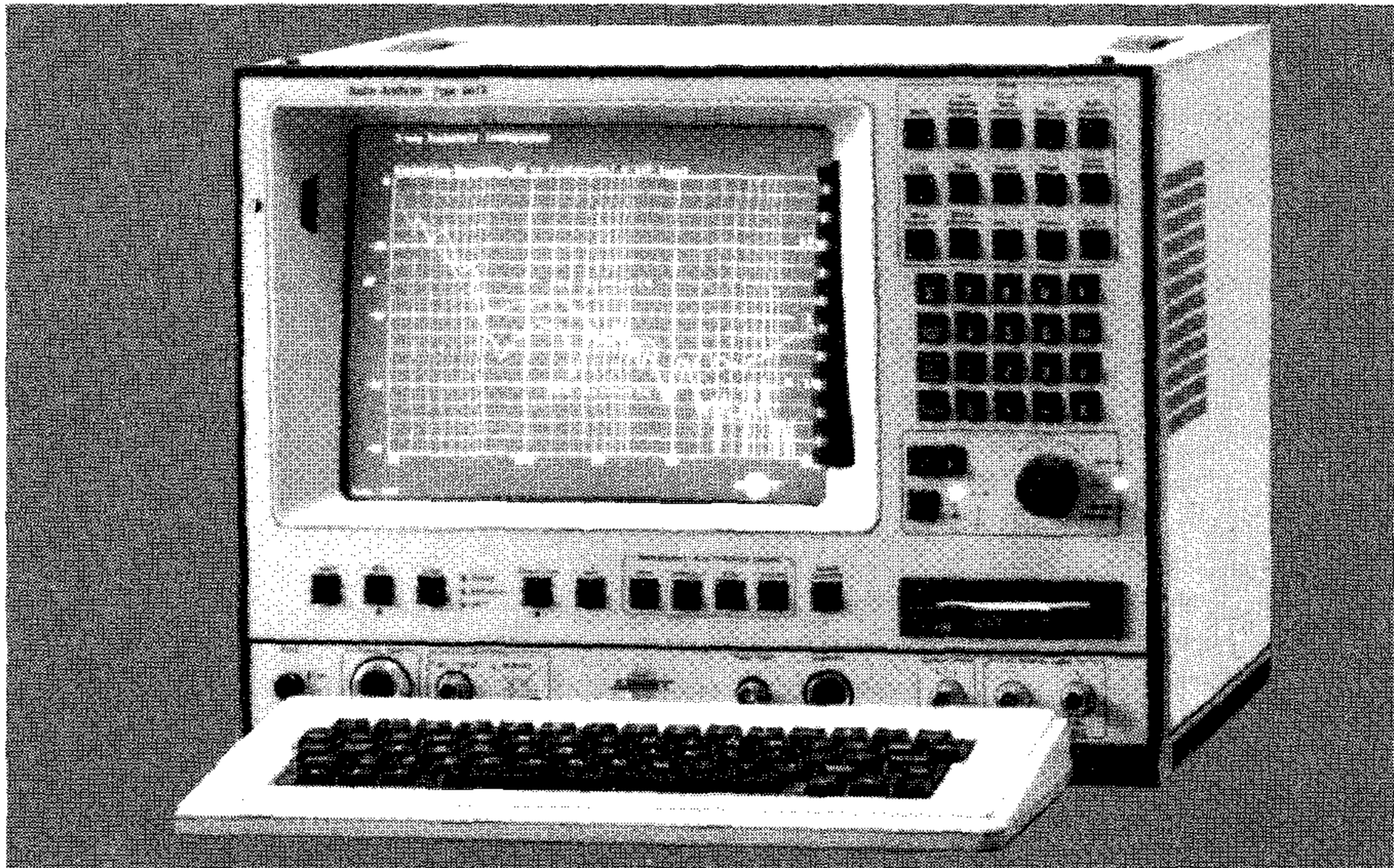
Fig. 28 The 2012 Audio Analyzer allows fast distortion measurements in an ordinary room without the need for an anechoic chamber
